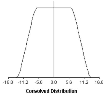
**An Approximate Utility Distribution.** Shown is the distribution for the sum of three uniformly distributed errors with equal means and where  $a > b > c$ . In the case depicted,  $c > a + b$ . Notice the similarity in form of the convolved distribution and the utility distribution discussed earlier.
