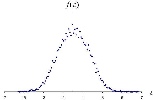
**Monte Carlo Simulation for the Distribution of the Sum of Two Uncorrelated Measurement Errors.** Shown is the distribution for a measurement error composed of a uniformly distributed error with bounding limit  $a = 2.0$  and a normally distributed error with a standard deviation of 1.0. The population standard deviation (standard uncertainty) is 1.5275. The standard deviation computed from the simulated distribution is 1.5238.
