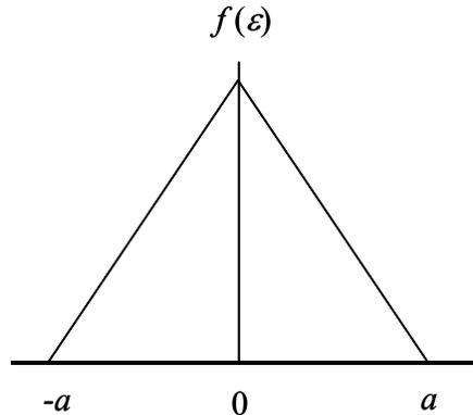
**The Triangular Distribution.** A distribution for linear combinations of two uniformly distributed variables with equal mean values and bounding limits.
