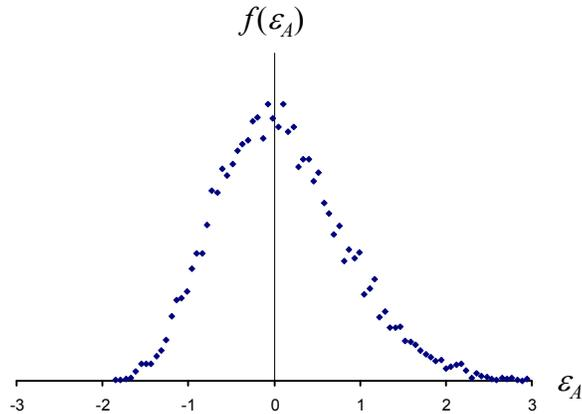
**Monte Carlo Simulation for the Distribution of Correlated Measurement Biases.** Shown is the distribution for the error in the measurement of a rectangular plate of length 1.0 and width 2.0. In constructing the distribution, 10,000 random normal deviates were simulated from a population with mean zero and standard deviation 0.25. The population standard deviation is 0.75. The standard deviation computed from the simulated distribution is 0.7544.
