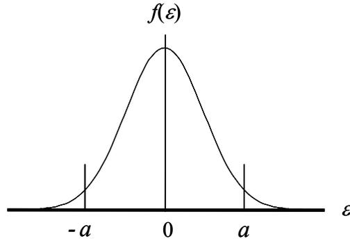
**The Normal Distribution.** Shown is a case where the error distribution mean value is zero. The limits  $\pm a$  are approximate 95% confidence limits.
