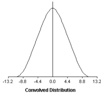
**An “Unbalanced” Uniform Convolution.** Shown is the distribution for the sum of three uniformly distributed errors with equal means and where  $a > b > c$ . In the case depicted,  $c < a + b$ . In this case, the convolved distribution appears to favor both the normal and triangular distributions.
