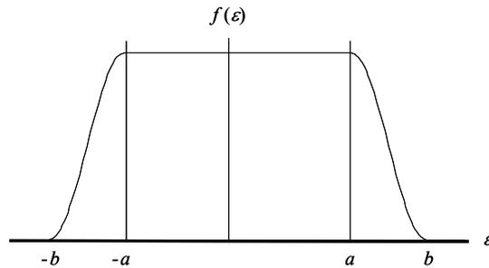
**The Utility Distribution.** The probability of occurrence is approximately uniform between the values  $\pm a$ , tapering off to zero at the limits  $\pm b$ .
