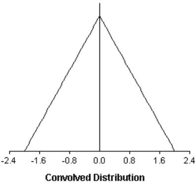
**The Triangular Distribution.** Shown is the distribution for the sum of two uniformly distributed errors with equal means and equal limits.
