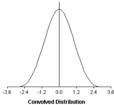
**Convolution of Uniform and Cosine Distributions.** Shown is the distribution for the sum of a uniformly distributed error and a an error that follows the cosine distribution. In the case depicted, mean values for both errors are zero and  $b = 2a$ .
