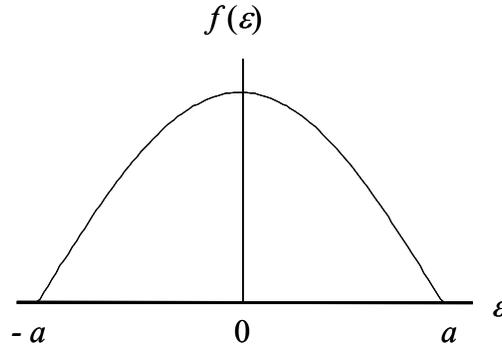
**The Half-Cosine Distribution.** Possesses a central tendency but exhibits a higher probability of occurrence near the minimum limiting values than either the cosine or the normal distribution.
