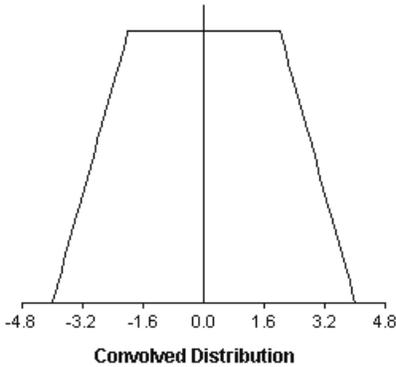
**The Trapezoidal Distribution.** Shown is the distribution for the sum of two uniformly distributed errors with equal means and where  $b > a$ . A freeware application was used to develop the graphic [ISG04b].
