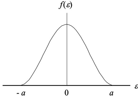
**The Cosine Distribution.** A 100% containment distribution with a central tendency and lacking discontinuities.
