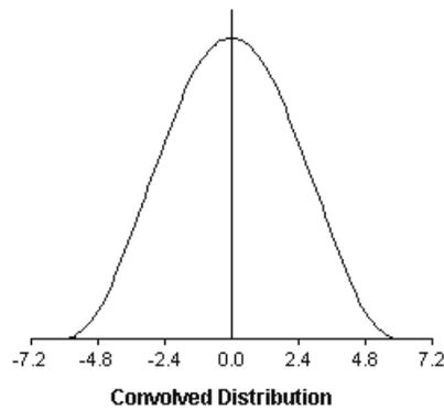
**A “Symmetric” Uniform Convolution.** Shown is the distribution for the sum of three uniformly distributed errors with equal means and where  $a > b > c$ . In the case depicted,  $c = a + b$ . In this case, the convolved distribution begins to take on the character of the normal distribution.
