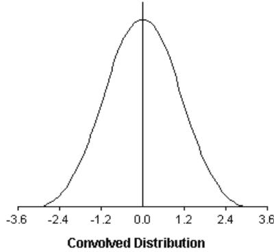
**A “Balanced” Uniform Convolution.** Shown is the distribution for the sum of three uniformly distributed errors with equal means and where  $a = b = c$ . In this case, the convolved distribution looks like a normal distribution cinched at the waist
