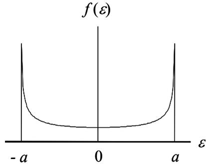
**The U Distribution.** The distribution is the pdf for sine waves of random phase incident on a plane.
