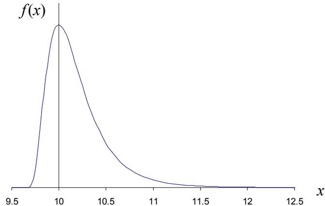
**The Lognormal Distribution.** Useful for describing distributions for parameters constrained by a physical limit or possessing asymmetric tolerances. The case shown is a "right-handed" distribution in which the mode value is greater than the physical limit.
