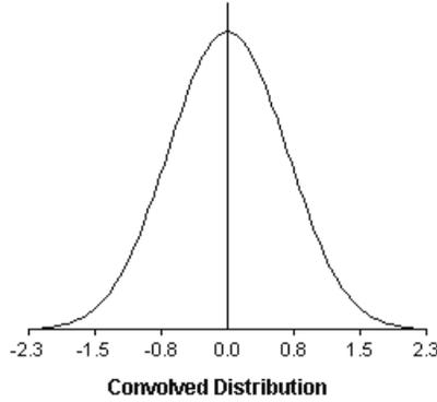
**Convolution of Uniformly and Normally Distributed Errors.** Shown is the distribution for the sum of a uniformly distributed error and a normally distributed error with mean values equal to zero. In the case depicted,  $u_1$  and  $u_2$  are equal.
