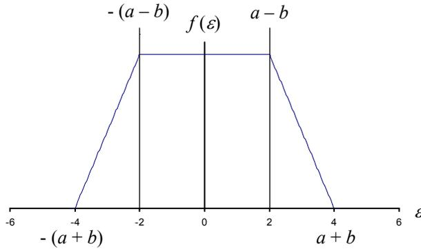
**Trapezoidal Distribution.** Shown is a distribution for the sum of two uniformly distributed variables with bound values  $a = 3$  and  $b = 1$ . The 100% containment limits are  $\pm (a + b)$  and the uniform density limits are  $\pm (a - b)$ .
