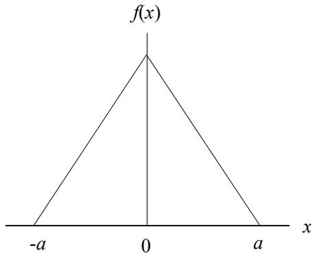
**The Triangular Distribution.** A distribution that sometimes applies to parameter values immediately following test or calibration.
