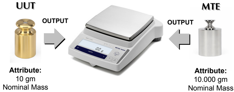
Figure 3. Scenario 3 – Measured values of the UUT and MTE attributes are compared using a comparator. The outputs are the weights of the masses.
